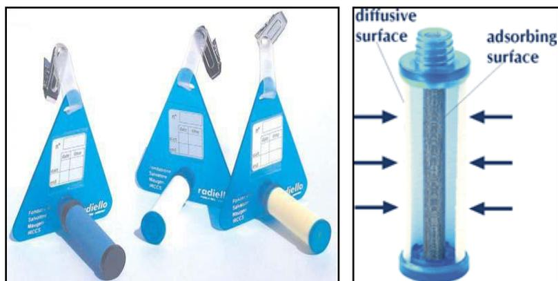
**Figure 1 : Passive Diffusion Tube Sampler**
